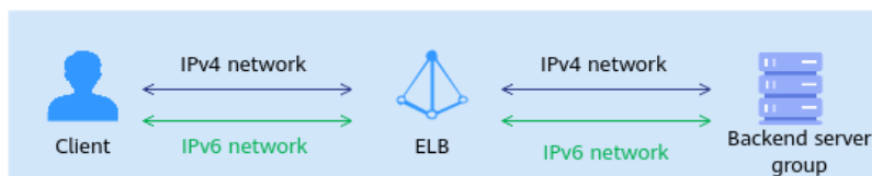
Figure 1-7 Service architecture with IPv4/IPv6 translation disabled for TCP and UDP listeners
